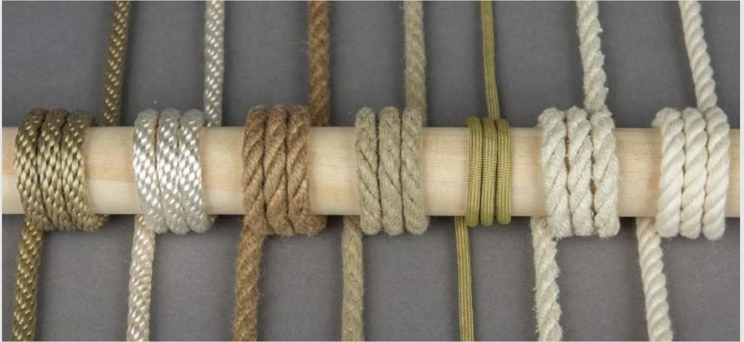
(From left to right) Multifilament Polypropylene (MFP), Nylon, Jute, Hemp, Paracord, Silk, Cotton
